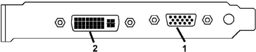
**Note** Please use the DVI-to-VGA adapter provided with your card to connect a second VGA monitor to the DVI connector (2).
