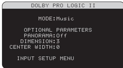
When Dolby Pro Logic II is selected as the default surround mode on the INPUT SETUP menu, there are additional settings and parameters to optimize the surround decoding for music or movie soundtracks. Dolby Pro Logic II uses matrix decoding algorithms to derive a center channel and surround channels from 2-channel source material.
